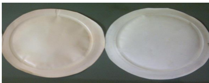
Figure 7: Changes in appearance of (a) Psf-LiOH, and (b) Psf-g7 membrane after filtration process
